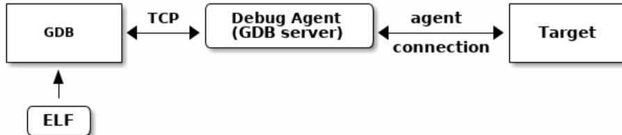
Fig. 10.1: Embedded Executable Debugging
