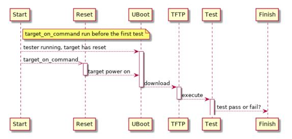
Fig. 11.6: Test Pass and Fail Sequences
