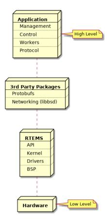
Fig. 9.1: Vertical Software Stack
