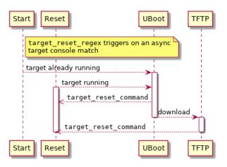
Fig. 11.8: Target Reset Filter Trigger
