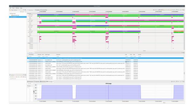
Fig. 12.5: Once a trace is opened, the main window shows you a couple of views, for example *Resources*, the trace log, and *CPU Usage*. The *Resources* view shows you the CPU utilization at a given time. A CPU may be idle, executing a thread, or executing an interrupt. The selected trace item in the trace log is shown as a vertical time bar in the *Resources* and *CPU Usage* view.
