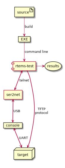
Fig. 11.5: RTEMS Tester using TFTP and U-Boot.
