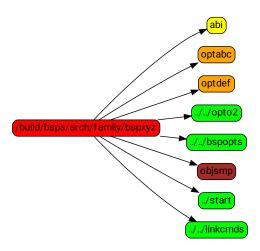
Fig. 10.3: This example shows a BSP family named *family* in the architecture *arch* which consists of only one base BSP named *xyz*. The BSP sources and installation information is contained in the spec:/build/bsps/arch/family/bspxyz BSP item. The items linked by the BSP item are shown using relative UIDs.
