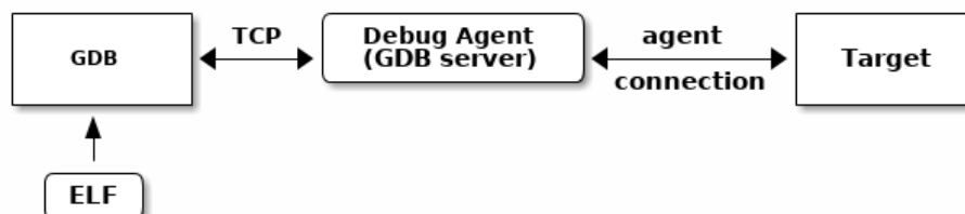
Fig. 10.1: Embedded Executable Debugging
