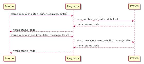
As illustrated in the preceding sequence diagram, the Source usually corresponds to application software reading a system input. The Source obtains a buffer from the Regulator instance and fills it with incoming data. The application explicitly obtaining a buffer and filling it in allows for zero copy operations on the Source side.
