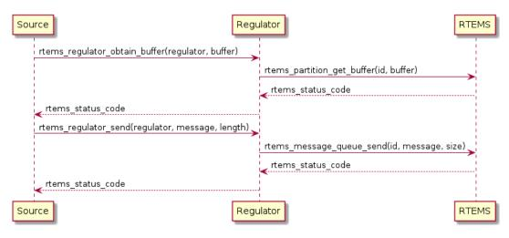
As illustrated in the preceding sequence diagram, the Source usually corresponds to application software reading a system input. The Source obtains a buffer from the Regulator instance and fills it with incoming data. The application explicitly obtaining a buffer and filling it in allows for zero copy operations on the Source side.
