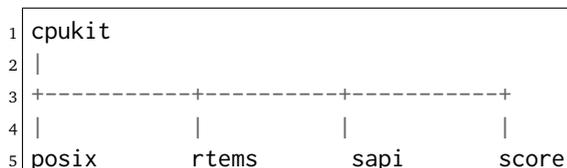
The `cpukit/` directory contains a set of subdirectories which contains the source files comprising the executive portion of the RTEMS development environment as well as portable support libraries such as support for the C Library and filesystems. The API specific and “SuperCore” (e.g. `score/` directory) source code files are separated into distinct directory trees.
