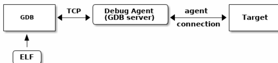
Fig. 9.3: Embedded Executable Debugging
