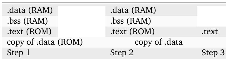
In Step 1, the program is linked together using the BSP linker script.
