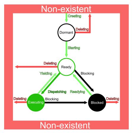
A task occupies the blocked state whenever it is unable to be scheduled to run. A running task may block itself or be blocked by other tasks in the system. The running task blocks itself through voluntary operations that cause the task to wait. The only way a task can block a task other than itself is with the rtems\_task\_suspend directive. A task enters the blocked state due to any of the following conditions:
