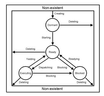
A task occupies the blocked state whenever it is unable to be scheduled to run. A running task may block itself or be blocked by other tasks in the system. The running task blocks itself through voluntary operations that cause the task to wait. The only way a task can block a task other than itself is with the rtems.task\_suspend directive. A task enters the blocked state due to any of the following conditions:
