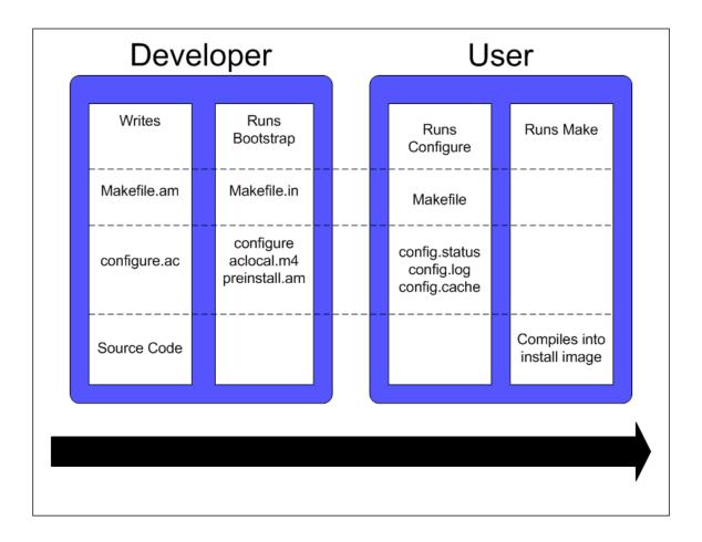
During the bootstrap phase, you are using the configure.ac and Makefile.am files as input to GNU autoconf and automake to generate a variety of files. This is done by running the bootstrap script found at the top of the RTEMS source tree.
