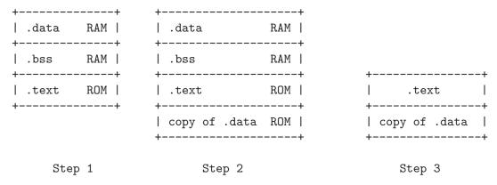
In Step 1, the program is linked together using the BSP linker script.
