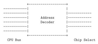
The Chip Select registers must be programmed such that they match the linkcmds settings. In the gen68340 BSP, ROM and RAM addresses can be found in both the linkcmds and initialization code, but this is not a great way to do this. It is better to define addresses in the linker script.
