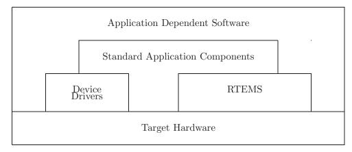
The RTEMS I/O interface manager provides an efficient tool for incorporating these hard-ware dependencies into the system while simultaneously providing a general mechanism to the application code that accesses them. A well designed real-time system can benefit from this architecture by building a rich library of standard application components which can be used repeatedly in other real-time projects.
