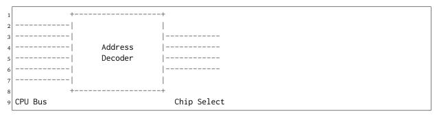
The Chip Select registers must be programmed such that they match the linkcmds settings. In the gen68340 BSP, ROM and RAM addresses can be found in both the linkcmds and initialization code, but this is not a great way to do this. It is better to define addresses in the linker script.
