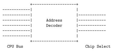
The Chip Select registers must be programmed such that they match the linkcmds settings. In the gen68340 BSP, ROM and RAM addresses can be found in both the linkcmds and initialization code, but this is not a great way to do this. It is better to define addresses in the linker script.
